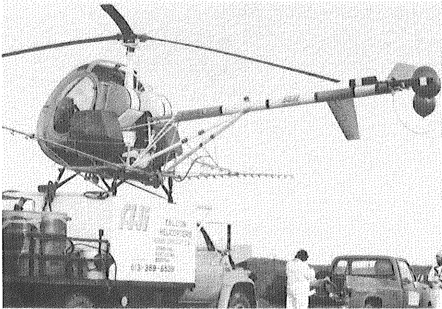
Falcon Hughes 300 with Agranautics spray kit. It rests on the Falcon nurse-rig.
